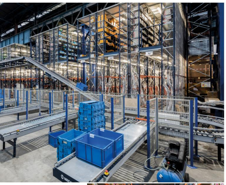
Racks with walkways take full advantage of the height of the distribution center to max out available space and provide greater storage capacity
