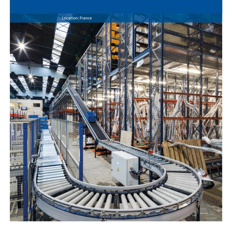
Automotive Factory Parts, an automobile spare parts distributor, owns a 1.24 acre modern logistics center in Gennevilliers (France), whose principal operation is the picking of online orders. Mecalux has provided the storage systems, including a circuit of conveyors that link all areas of the installation, so that picking is carried out faster.
