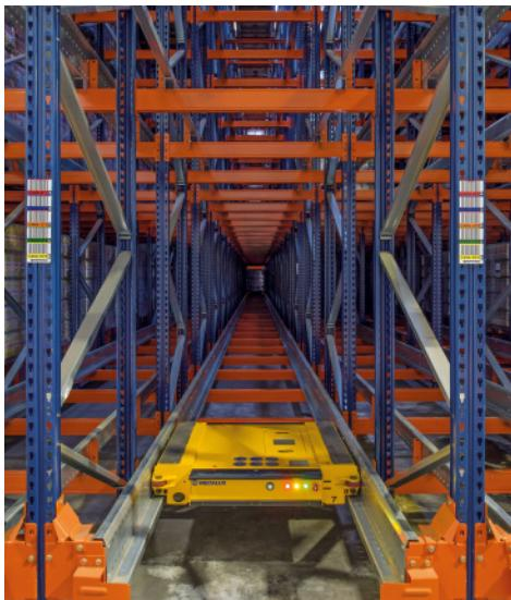
in Europe (mainly, France, Germany and Spain). Operators carry a handheld control tablet (with Wi-Fi) to run the Pallet Shuttles remotely. The tablet's monitor is highly-intuitive and requires no specialised training to use. Then, from the device, workers can execute numerous apps and functions like choosing how many pallets must be inserted or extracted or carrying out an inventory count.
