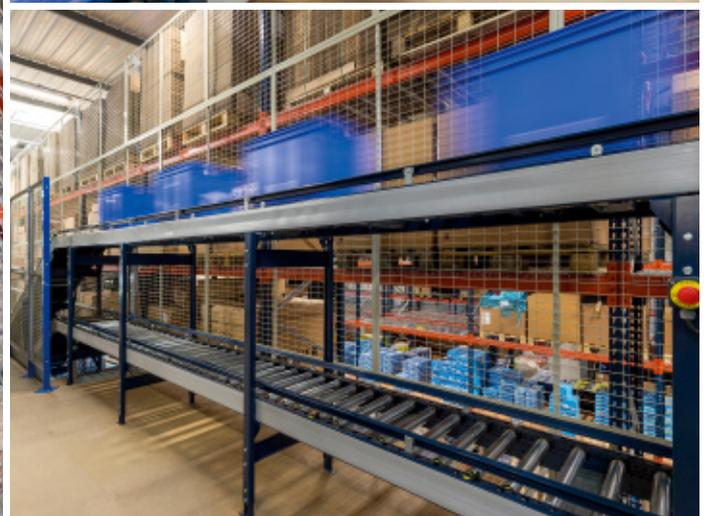
A combination of roller and belt conveyors run along the route. The inclined belts are very useful in dealing with slopes in the warehouse.
