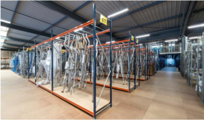
Bulky products are deposited in the racks best suited to facilitating their management. For example, exhaust pipes are placed in racks and a portion of these pieces rest on a chipboard shelf surface.
