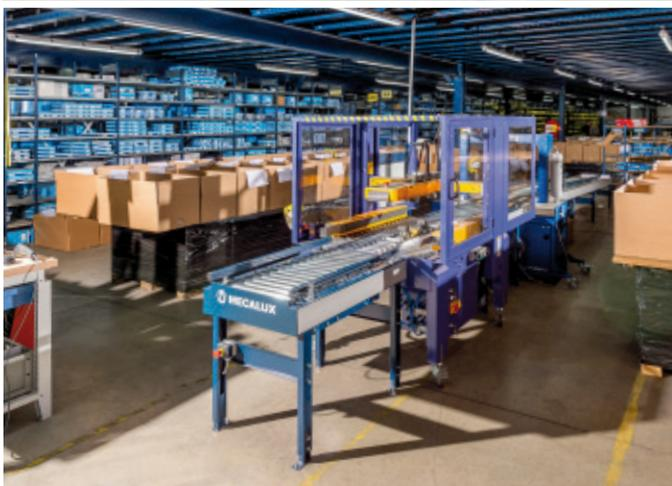
Van Heck Interpieces, an automotive spare parts distribution business, owns a 4,000 m<sup>2</sup> warehouse on the outskirts of Lyon (France). There, all the storage systems have been supplied by Mecalux: a two-level high mezzanine in addition to the ground floor, storage for picking and a conveyor system that connects all the levels. Altogether, these solutions provide streamlined picking and are capable of organising products of different sizes, volumes and turnovers.
