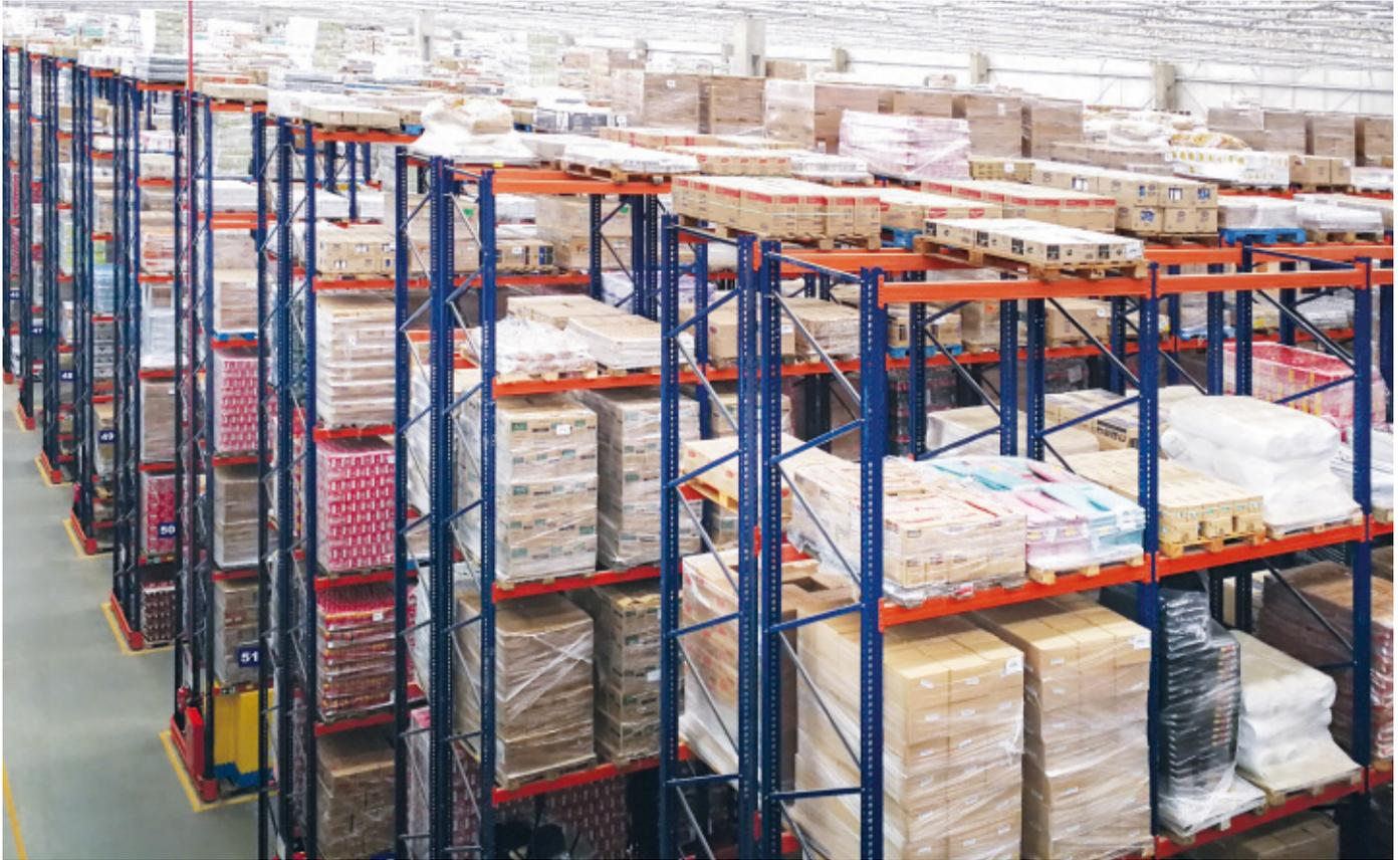
The products in greatest demand are placed at the ends of the aisles, closest to the loading bays, to speed up their movement in and out of the warehouse
