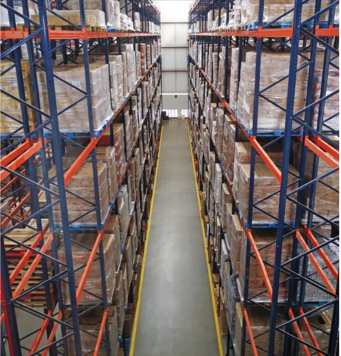
The Brazilian supermarket Super Nosso has opened a new 25,000 m<sup>2</sup> distribution centre in Contagem (in the state of Minas Gerais). Mecalux has equipped it with 15 m high pallet racks with a total storage capacity of 37,800 pallets. These offer direct access to the products, which simplifies preparing the 3,000 daily customer orders.
