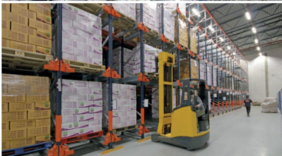
Firat Food, a food and beverage wholesaler, has reorganized operations in its French warehouse to streamline picking. Mecalux supplied selective pallet racking, the high-density Pallet Shuttle system and a roller conveyor, which joins the different areas that make up the installation.
