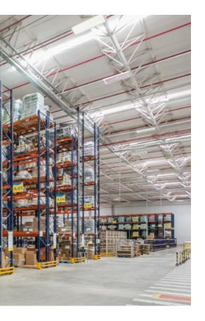
There is a transversal aisle enabled in the central area that crosses the storage aisles, facilitating the flow between the different zones in this area. The width of this aisle enables the circulation of two handling machines at the same time.
