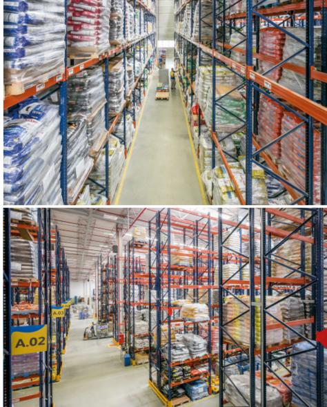
With a height of 31', the selective pallet racks in this area can store 3,808 pallets of 39" x 48" with a maximum unit weight of 1.38 t
