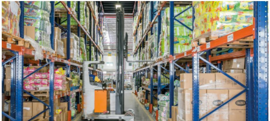
There is a transversal aisle enabled in the central area that crosses the storage aisles, facilitating the flow between the different zones in this area. The width of this aisle enables the circulation of two handling machines at the same time.
