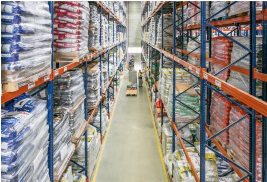
With a height of 31', the selective pallet racks in this area can store 3,808 pallets of 39" x 48" with a maximum unit weight of 1.38 t
