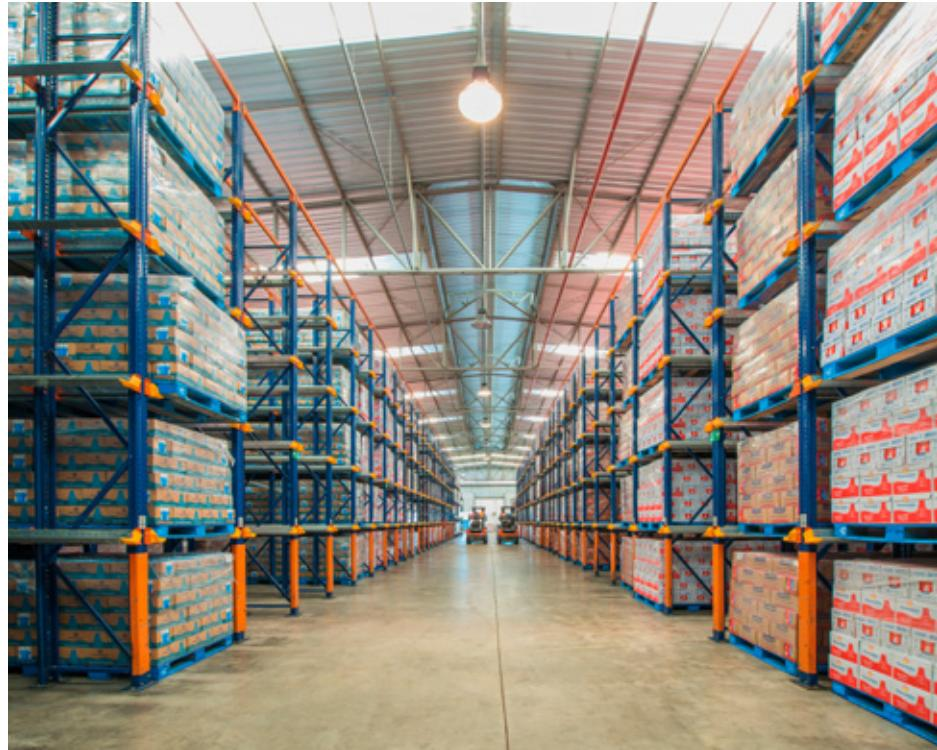
Operators, aided by reach trucks, enter the inner lanes with the load perched above the level where it must be deposited. Both loading and unloading of the goods is done in the same aisle, but in reverse.
