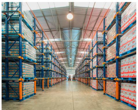
Operators, aided by reach trucks, enter the inner lanes with the load perched above the level where it must be deposited. Both loading and unloading of the goods is done in the same aisle, but in reverse.
