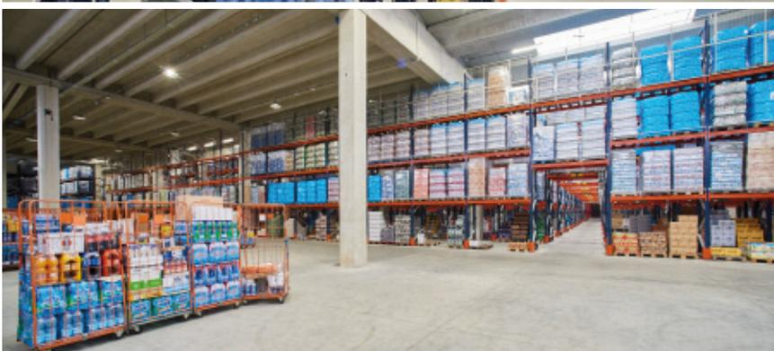
The warehouse of the Italian company Centro 3A SPA, equipped with Mecalux selective pallet racks, has capacity for 7,826 pallets. This system facilitates direct access to the goods, which streamlines the storage and picking tasks.
