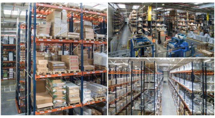
The pallet racks installed in Sectors 1, 2, 3 and 4 have an overall capacity for 35,000 pallets filled with a large variety of products in multiple sizes.
