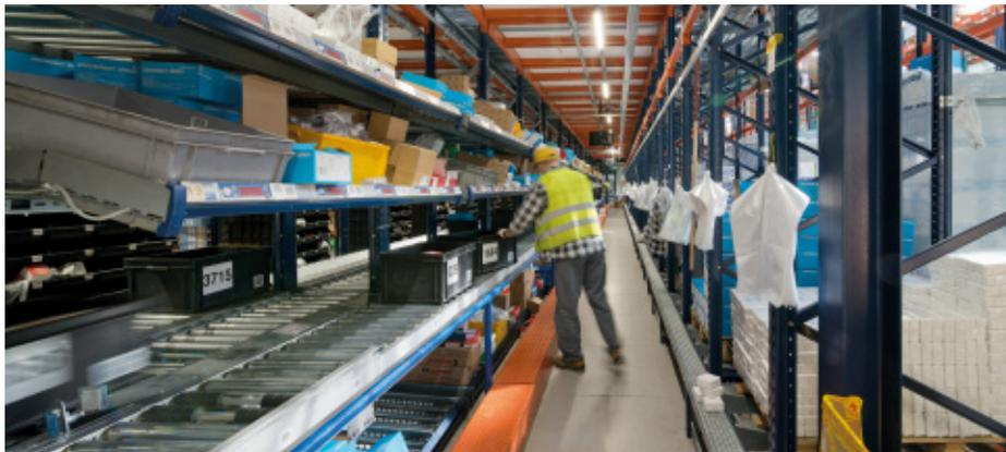
The pick module consists of flow racks for pallets and boxes, racks with shelves and a conveyor circuit that creates two order prep areas on each floor
