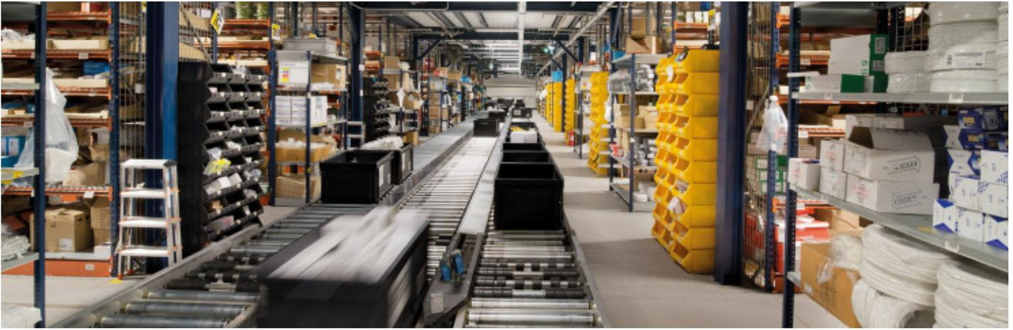
Rack levels are made out of perforated shelves that, in addition to having a high load capacity, favor the flow of water in case the fire safety system is activated.
