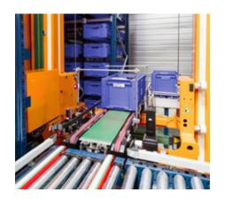
The miniload incorporates a double box extraction system in its cradle, able to handle two boxes at the same time and can even access the second position of each location. It has a fork and two moving joists able to pick the boxes up from either one side of the aisle or the other.
