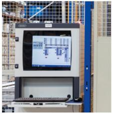
The Galileo control module is responsible for directing the maneuvers the moving devices must perform in the installation, such as the miniload stacker cranes and conveyors
