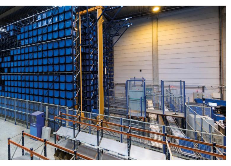
Twin-mast miniload stacker cranes move along each aisle, tasked with managing the inputs and outputs of the goods. These machines operate at a travel speed of 820 ft/min and 295 ft/min when elevated.
