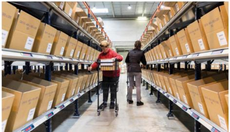
Each location on the racks is equipped with a display that lights up and shows the number of required items. The operators walk the aisles, placing the products in the boxes signaled by the put-to-light devices, then press the indicator to confirm that they have performed the action.
