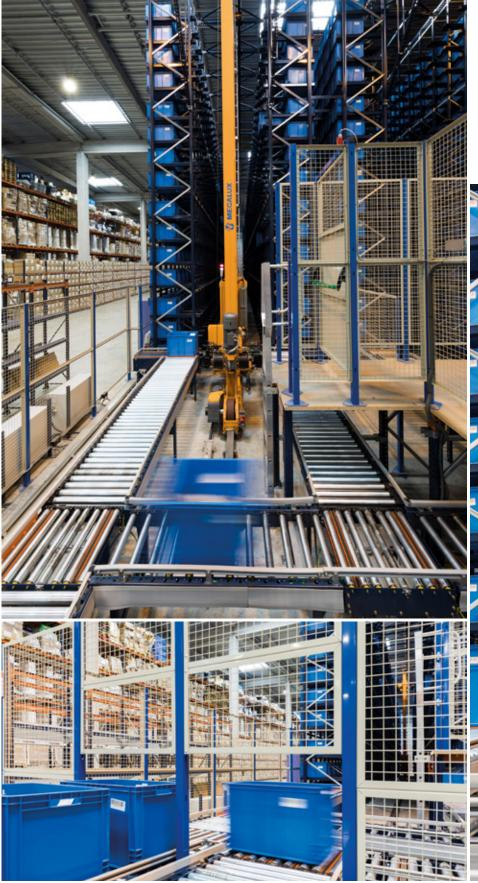
At the front of the automated warehouse are three picking stations where orders are prepared according to the product-to-person principle, in other words, the stacker cranes take the merchandise directly to the operators. To do this, they place the boxes on the conveyors, which automatically lead to the picking stations.
