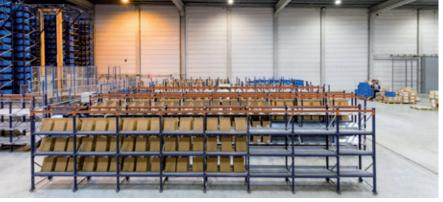
The Groupe Rand distribution center in Longueil Sainte Marie (France) stands out for its picking flexibility and agility. The installation supplied by Mecalux consists of an AS/RS for boxes with a storage capacity of more than 15,300 boxes, selective pallet racking and racks with put-to-light devices. These classify merchandise several orders at a time, without the usual errors stemming from manual management.
