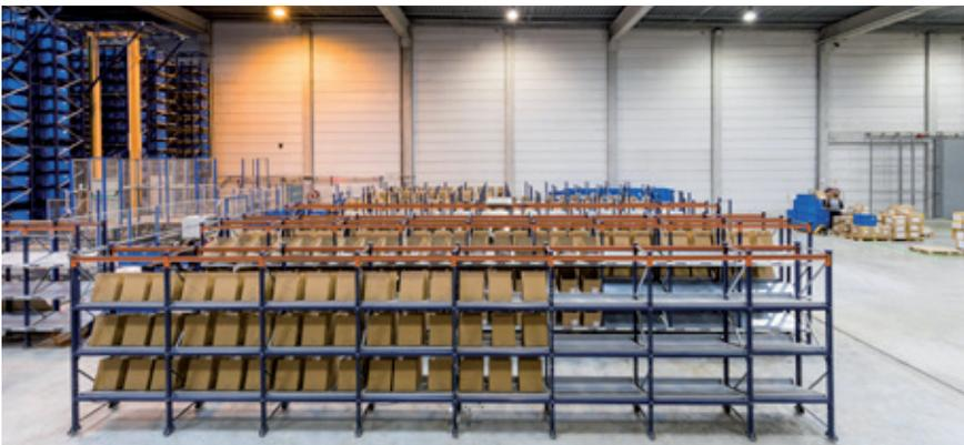
The Groupe Rand distribution center in Longueil Sainte Marie (France) stands out for its picking flexibility and agility. The installation supplied by Mecalux consists of an AS/RS for boxes with a storage capacity of more than 15,300 boxes, selective pallet racking and racks with put-to-light devices. These classify merchandise several orders at a time, without the usual errors stemming from manual management.
