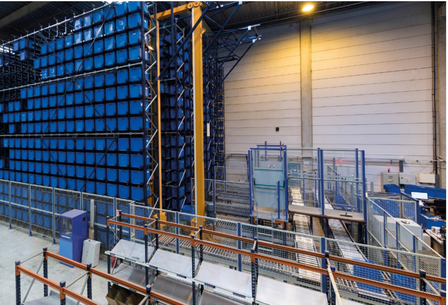
Twin-mast miniload stacker cranes move along each aisle, tasked with managing the inputs and outputs of the goods. These machines operate at a travel speed of 820 ft/min and 295 ft/min when elevated.
