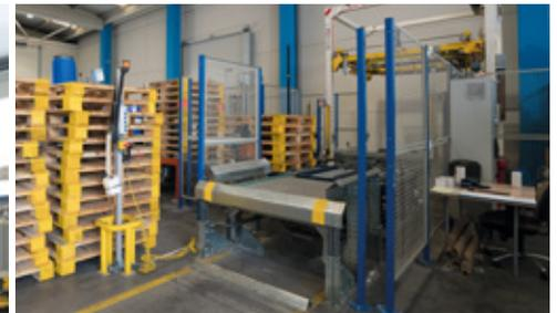
The pallets must pass a checkpoint where the weight, size and condition of the goods are verified
