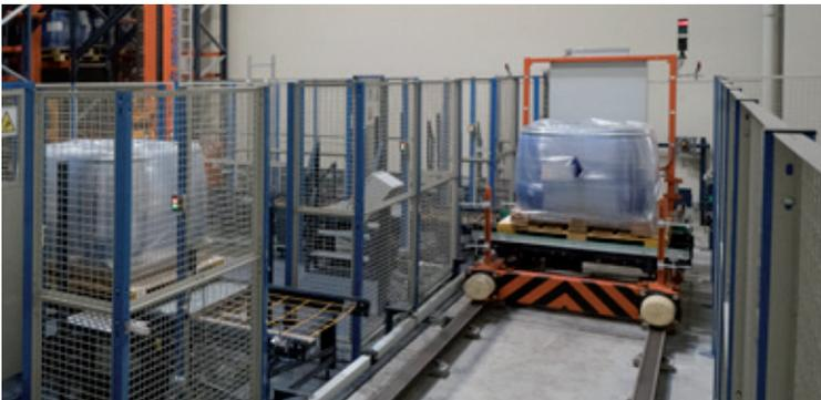
Mecalux has built an Automated Storage & Retrieval System (AS/RS) for the chemical company Trumpler, consisting of two double aisles with double-depth racks on both sides. Two twin-mast stacker cranes with telescopic forks are in charge of introducing and removing the goods from their corresponding locations. This facility, located in Barcelona, has a 2,512 pallet capacity and the entire operation is supervised by the Easy WMS warehouse management system from Mecalux.
