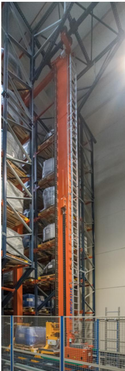
AS/RS stacker cranes have double-depth telescopic forks that help to deposit and extract loads from secondary locations on the racks
